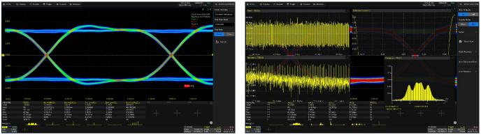
Supports eye diagram and jitter analysis/measurement. It can automatically extract the embedded reference clock from serial data and create the eye diagram. Measurement on multiple eye/jitter parameters is provided. Mask test on eye diagrams is supported
