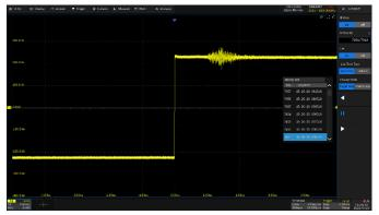
History function can record up to 124,000 frames of waveforms. The recording is executed automatically so that the customer can playback the history waveforms at any time to observe unusual events and quickly locate the area of interest using the cursors or measurements. The failed frames of the Mask Test can be stored as history
