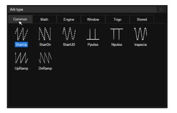
The oscilloscope can control the built-in waveform generator to output waveform with up to 50 MHz frequency and  $\pm$ 3 V amplitude. Six basic waveforms plus multiple types of arbitrary waveforms are built-in
